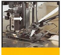
OPTOELECTRONIC SENSOR Integrated into the sewing parts, sensor controls the "FAST ACTION TAPE CUTTER" so it operates as close as possible to the needle for accurate cutting.
