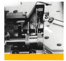
**Quicker threading** The cast-off plate easily swings up and out of the way, making threading faster and easier.
