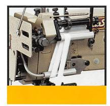
ELASTIC METERING DEVICE The top metering device maintains the desired tension automatically at all times, independently of stitch length and machine speed. Available in both single and two-stage versions. Two-stage version has engageable, disengageable tension during sewing.
